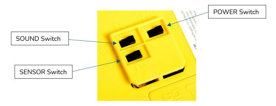
As the diagram shows, there are three switches located underneath Bee-Bot:
