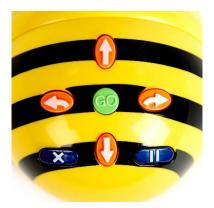
As you can see from the diagram above, Bee-Bot has a set of coloured, command buttons on the top of its case:
