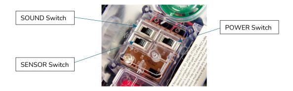
As the diagram shows, there are three switches located underneath Blue-Bot:
