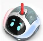
Loti-Bot is a member of the TTS Bot Family, featuring programmable movement, highly accurate drawing capabilities and a variety of inputs and outputs.
