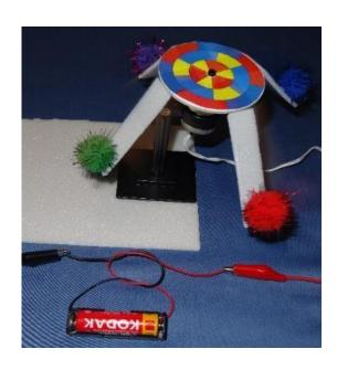
N.B. If you are dismantling this model to use for the next module then try to remove the motor stand carefully from the polystyrene base, so that you can re-use the base in module 4.
